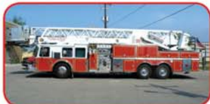
1990 Grumman / HME 102' Platform Detroit 475 HP Diesel Allison Automatic Transmission Waterous 1500 GPM Pump 200 Gallon Poly Tank Onan 7.5KW Generator
