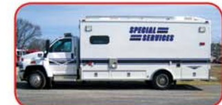
2006 Chevy / Pierce Command Center Duramax Diesel, Allison Automatic 10KW Diesel Generator 1/3" CCD Telescoping Camera Sink, Refrigerator, Microwave 2 - 20" Flat Panel Televisions
