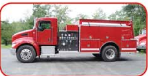
2009 Kenworth Commercial Pumper Diesel Engine, Allison Automatic Hale 1250 GPM Side-Mount Pump 750 Gallon Poly Tank Foam Capable Pre-2010 Emissions
