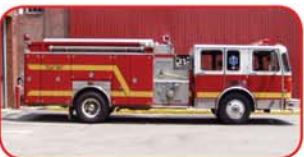
1993 Ferrara / Spartan Rescue Pumper Cummins 300 HP Diesel Engine Allison Automatic Transmission Hale 1500 GPM Side-Mount Pump 1000 Gallon Poly Tank Feecon Around-the-Pump Foam System
