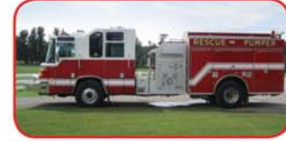
2000 Pierce Quantum Rescue Pumper Detroit Series 60 470 HP Diesel Allison HD4060 Automatic Hale 1500 GPM Top-Mount Pump 750 Gallon Poly Tank
