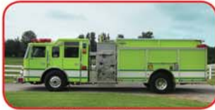
2000 Pierce Dash Pumper Detroit Series 50 350 HP Diesel Allison MD3066R Automatic Waterous 1250 GPM Pump 1000 Gallon Poly Tank Around the Pump Foam System
