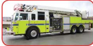
2001 Pierce Dash 75' Quint Detroit Diesel, Allison Automatic Hale QMAX 2250 GPM Pump FoamPro 1600 Class A System 480 Gallon Poly Tank AMPS 15 KW Hydraulic Generator
