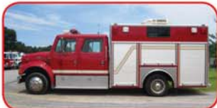
1996 Kenco / Int'l Medium-Duty Rescue Navistar 175 HP Diesel Engine Allison MT643 Automatic Transmission PTO-Driven Generator WillBurt Light Tower w/ 4-1500W Lights
