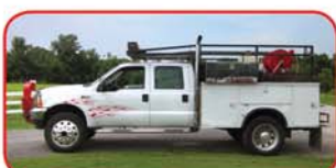
2001 Ford F-550 4x4 Brush Truck Ford 7.3L Powerstroke Diesel Ford 2711F Manual 100 GPM Pump 300 Gallon Polypropylene Tank Foam-It System with 20 Gallon Tank
