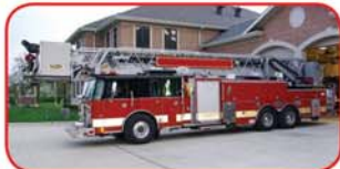
1998 Pierce 100' Platform Diesel Engine Allison Automatic Transmission Waterous 1250 GPM Pump 400 Gallon Poly Tank
