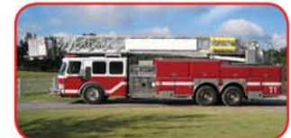
1991 E-One Hurricane 95' Platform Detroit 6V92TA 300 HP Diesel Allison MD3060 Automatic Hale QSMG 1250 GPM Pump 300 Gallon Poly Tank
