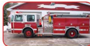
1993 E-One Custom Pumper Cummins 300 HP Diesel Engine Allison MD3060 Automatic Hale 1250 Side-Mount Pump Robwen on Board Foam System 1000 Gallon Poly Tank
