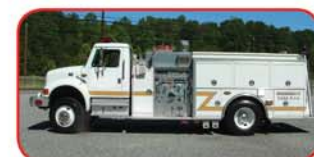
1999 KME / International 4x4 Pumper International 250 HP Diesel Allison Automatic Transmission Hale 1250 GPM Side-Mount Pump 500 Gallon Poly Tank 3300 Watt Diesel Generator
