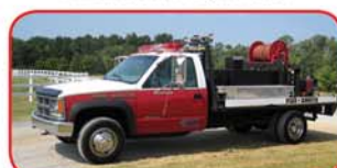
1999 Chevy 1-Ton 4x4 Brush Truck Gas Engine, Automatic Transmission 200 GPM Gas-Powered Pump 250 Gallon Tank 5KW Generator
