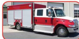
2009 Taylor Made / Int'l Medium Rescue Int'l MaxxForce 225 HP Diesel Allison 2200EVS Automatic Harrison 10KW Hydraulic Generator 3 - Portable Winch Receivers
