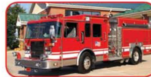
1995 Spartan / Saulsbury Pumper Diesel Engine Automatic Transmission 1250 GPM Side-Mount Pump 1000 Gallon Poly Tank
