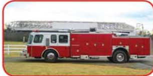
1995 E-One Hurricane 110' Aerial Detroit 6V92TA Diesel Engine Allison HT 740 Automatic Piped Waterway Fabco 8KW PTO-Driven Generator
