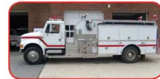
1991 Ferrara / Int'l Pumper / Tanker Navistar 270 HP Diesel Engine Allison Automatic Transmission Darley 1000 GPM Top-Mount Pump 1500 Gallon Tank
