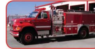
1995 Ford / E-One Pumper Cummins 8.3L 250 HP Diesel Allison MD3060 Automatic Hale 1250 GPM Side-Mount Pump 1000 Gallon Poly Tank
