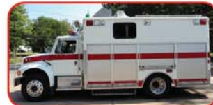
1993 International Medium Rescue Navistar Diesel, Allison Automatic Waterous 300 GPM PTO-Driven Pump 300 Gallon Poly Tank Winco 25KW PTO-Driven Generator Wilburt 6000W Light Tower
