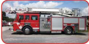
2002 American LaFrance 75' Quint Cummins ISM 400HP Diesel Allison MD3060P Automatic Hale 1250 GPM Side-Mount Pump 400 Gallon Poly Tank 6KW Hydraulic PTO-Driven Generator
