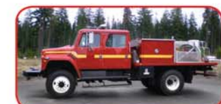
1987 International 4x4 Wildland Unit Diesel Engine, Allison Automatic Deutz-Ruggerini Diesel-Powered Pump Robwen Class A Foam System 750 Gallon Water Tank 40 Gallon Foam Tank
