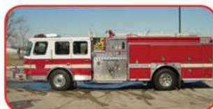
1999 E-One Cyclone Rescue Pumper Cummins ISM 320 HP Diesel Allison MD3060 Automatic Hale 1250 GPM Side-Mount Pump 500 Gallon Poly Tank
