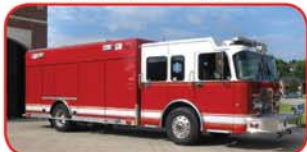
2005 Hackney / Spartan Heavy Rescue Cummins ISC 330 HP Diesel Allison 3000EVS Automatic Onan 25KW PTO Generator Willburt 9000W Light Tower
