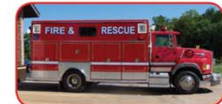
1993 EVI / Ford Walk-In Heavy Rescue Cummins Diesel, Allison Automatic 25KW PTO Generator 6-bottle 6,000 psi Cascade System Command Desk Area
