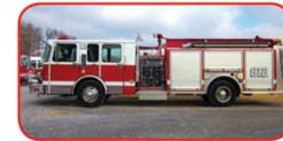
1997 Southern Coach Pumper Cummins C8.3 325 HP Diesel Allison MD 3060 Automatic Hale 1500 GPM Side-Mount Pump 750 Gallon Poly Tank
