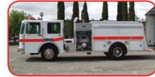
1992 Beck / Spartan Custom Pumper Cummins 8.3L Diesel Engine Allison Automatic Transmission Darley 1250 GPM Pump 500 Gallon Tank
