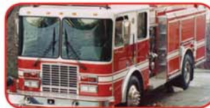
1997 Darley / HME Rescue Pumper Cummins C8.3 325 HP Diesel Allison MD 3060 Automatic Darley 1500 GPM Side-Mount Pump 750 Gallon Poly Tank CAF System with 30-Gallon Foam Cell
