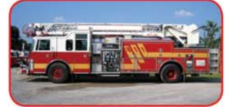
1996 Pierce Lance 75' Quint Detroit 8V92TA 500 HP Diesel Allison HD4060PR Automatic Hale QSMG150 1500 GPM Pump 300 Gallon Poly Tank Onan 6KW Diesel Generator
