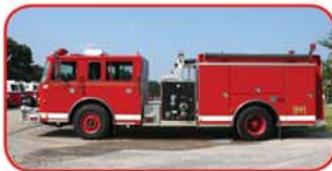
1998 Pierce Saber Custom Pumper Cummins 8.3L 325 HP Diesel Allison MD3060 Automatic 1250 GPM Waterous Top-Mount Pump 1000 Gallon Poly Tank
