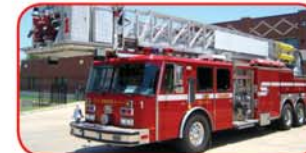
1994 E-One Hurricane 95' Platform Detroit 8V92 450 HP Diesel Allison HT740 Automatic Waterous 2000 GPM Pump 200 Gallon Poly Tank Foam System
